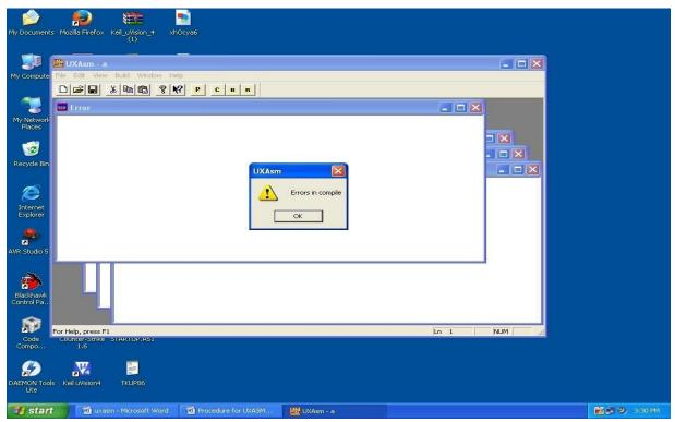
10. If any errors, Fix the errors, click on "OK" and click on "B" to build the program
