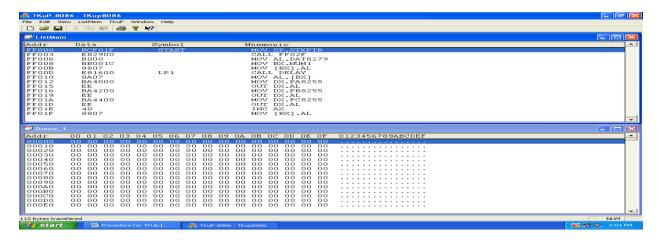
10. To verify the output, change the "SW-PP PROGRAM" switch to execution mode and verify output
